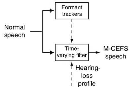
Fig. 1. Schematic of the M-CEFS amplification system.
